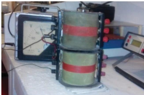
Photo 2 Dehydration emulsion under conditions of high-frequency magnetic field BSU Technological Faculty, in petroleum research laboratory conditions.
