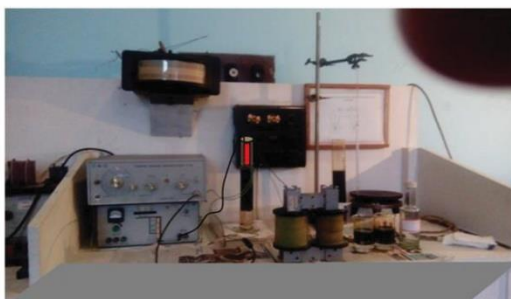
Photo 1 Demulsification of oil emulsion when exposed to a magnetic field in the range of 20-50 hertz, in the presence of demulsifier rAlkan - 202. Method 1.
